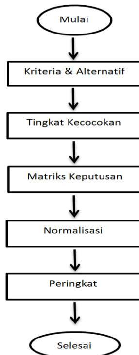
Gambar 3.2. Diagram Alur Simple Additive Weighting (SAW)
