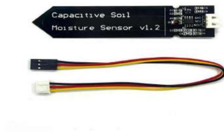
Gambar 2. 1 Sensor Capaitive Soil Sumber: (Suryana, 2021,p.4)
