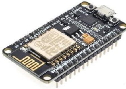
Gambar 2.3 ESP8266/NodeMCU
