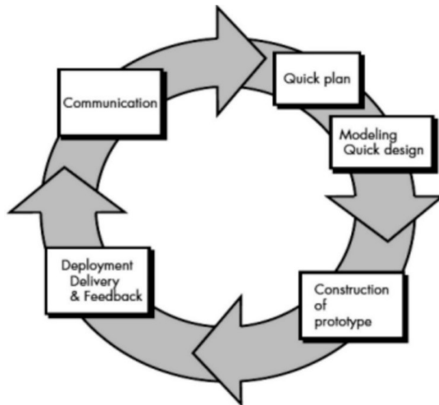
Gambar 3.3 Metode Prototype Sumber (Roger S, Pressman, 2012 , p. 51)
