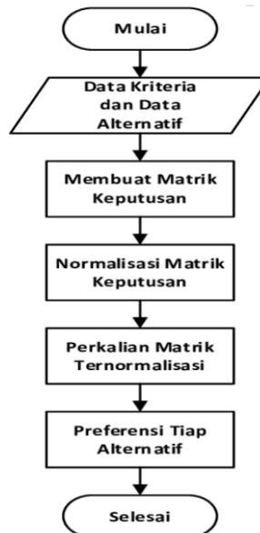
**Gambar 3. 2 Flowchart Simple Additive Weighting (SAW)**
